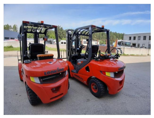
New Lpg3000 gas/petrol forklift. (Located in Vvn warehouse and can be received within 1 day) Other models: with diesel engine, gas (LPG) engine, electric engine.
